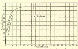
Fig. 9.—Typical characteristic curve of a lagged-type demand meter made for a 15-minute time interval.
